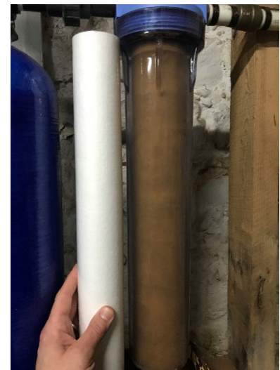
Figure 7: Discoloration in water filter following the January 24, 2020 water main break at Main St and Delevan Ave.
