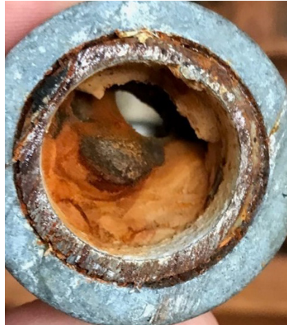
Figure 4: Note the scale in this section of pipe that was removed from our 1892 home in the Parkside neighborhood of North Buffalo when the water service line was replaced in July, 2016.
